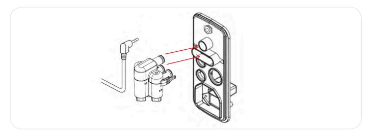
7. Insert 3.5mm sensor cable plug into the pump interface panel jack.
