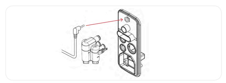
8. Connect the mains power cable to the pump ensuring that the power switch remains switched OFF
